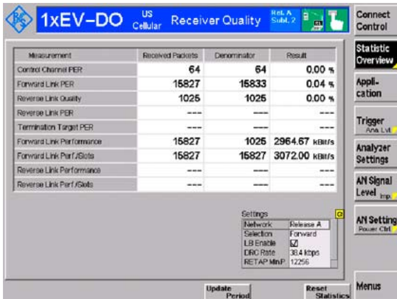
The Statistic Overview display of the Receiver Quality application, showing the DUT's received packet errors during a RETAP connection. The achieved throughput (net rate) is calculated and displayed as Forward Link Performance.
